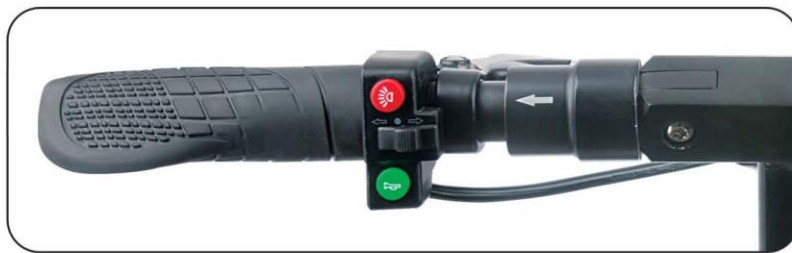
LED front light/speed control switch (left fast/right slow)/horn switch
